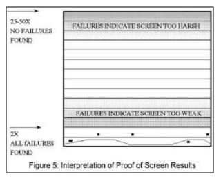
one or two cycles through the screen will precipitate all the seeded failures. This will yield a short, efficient screen, typically lasting less than 2 hours. As Figure 5 shows, if seeded failures are not precipitated until several passes through the screen, then the severity of the screen should be increased. This part of the PoS verifies that the screen will reliably find defects.
