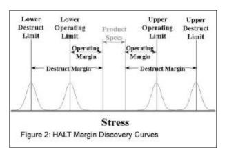
failure is seen, then it doesn't matter where in that distribution the unit under test falls – the failure mode will be detected. If the tail of that distribution happens to fall in the operating specifications, then the failure mode would have been an out-of-box failure mode on some fraction of your products. By doing HALT and stressing to failure, you will find the failure mode without having to hope that your sample size is big enough to exhibit the failure within operating specifications.
