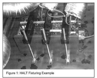
well as to improve the transmission of the low frequency energy, the product is set up on aluminum uchannel rather than being placed directly on the table top. The u-channel across the top of the product and the all-thread rod and nuts clamp the product to the table.
